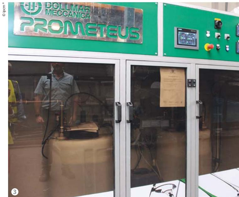
**Figure 3: DN Chemicals' Prometeus pre-treatment line for the application of nanotech products.**
