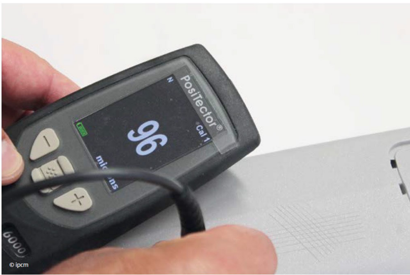
The coated products are subjected to strict quality controls using feeler gauges (pictured), gloss meters, and spectrophotometers.
