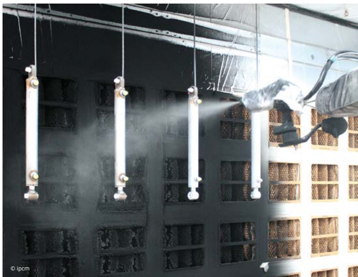
Paint application with an articulated robot.
