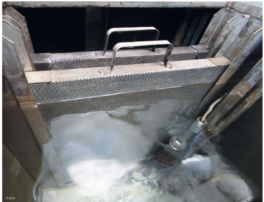
The entrance to the pre-treatment tunnel and one of its tanks.
