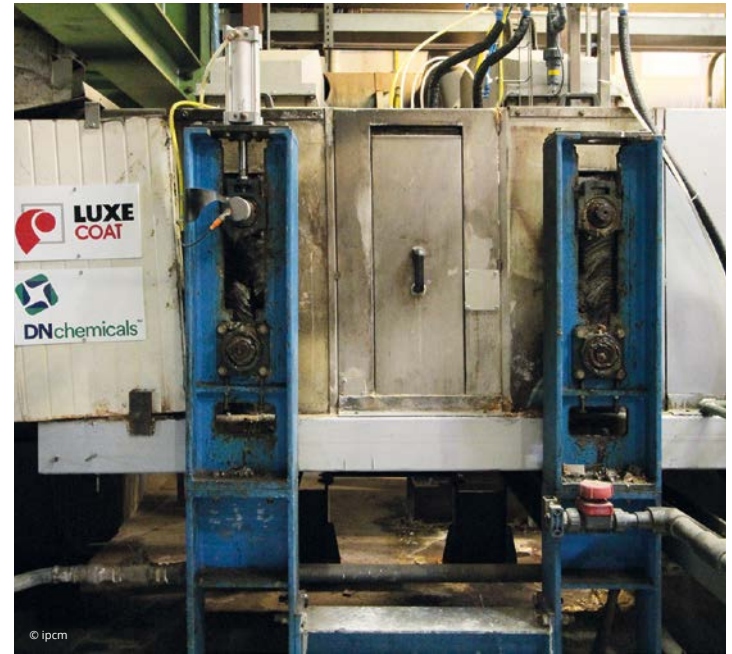
The two spraying bars of the nebulization module installed at the chromium-free nanotechnology conversion stage, supplied by DN Chemicals.
