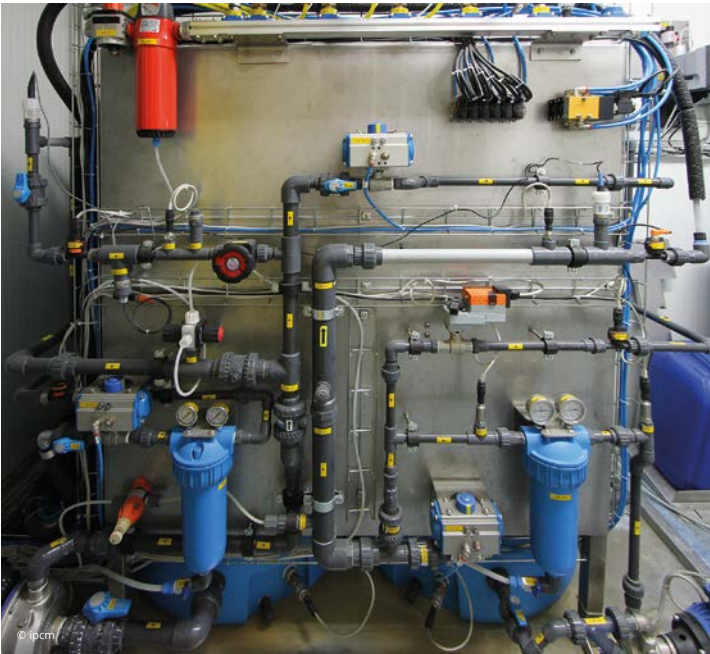
The Soft Rain device's circuit that feeds the ever-fresh passivation product to the spraying bars.
