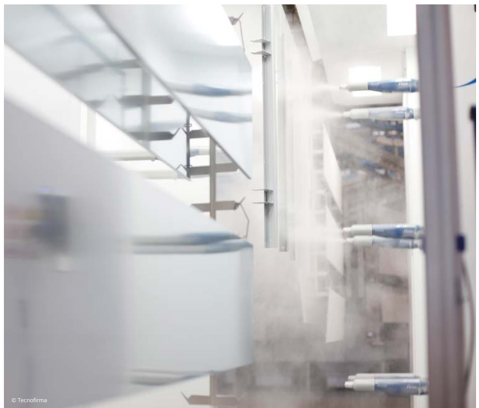
A phase of the coating application.
