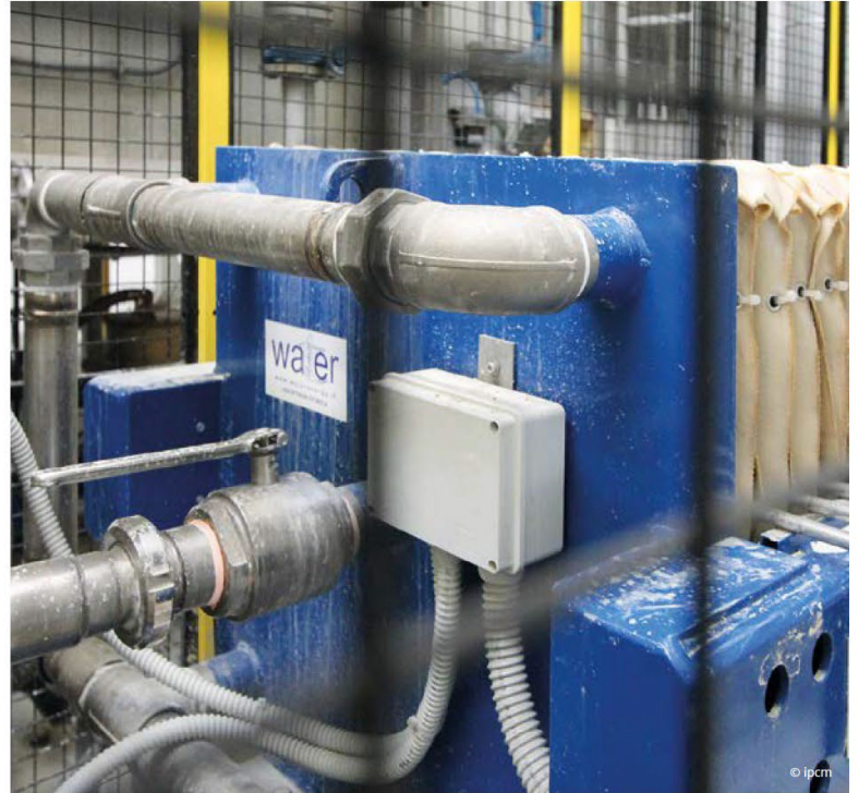
The detail of the filter press installed by Water Energy.
